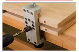
Once drilling is complete, loosen the knobs on the jig. Move jig to the next desired location and repeat steps 1 - 4 of this section until all of your holes are drilled. Step 5
