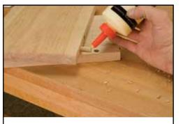
Once all of your holes are drilled apply glue to dowels and you are ready to assemble your joint.
