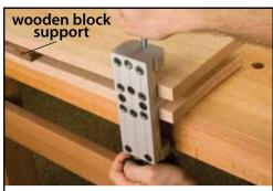
Once your boards are aligned, secure both stock pieces to the jig using the dowel jig knobs.
