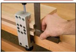
Place the stock pieces to be drilled into the dowel jig as shown in photo above. Both boards should be laying down horizontally. Use a square to ensure the both pieces are aligned correctly.
