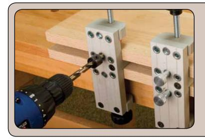
By adding a second Peachtree Dowel Jig (sold separately) you will be able to use the alignment pins, which are perfect for keeping your stock in place while you shift or slide the second dowel jig into position. Once your initial holes are drilled, insert the appropriate alignment pins into those two holes. Now, loosen the second dowel jig and slide it into position and secure. You are now ready to drill your second set of holes. Using a second jig cuts your drilling and setup time in half.
