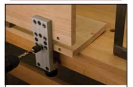
Once drilling is complete, loosen the knobs on the jig. Move jig to the next desired location and repeat steps 1 - 4 of this section until all of your holes are drilled. Step 5
